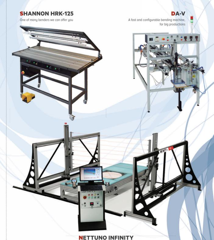
The Infinity Series consists of a range of computerized machines which, by using a "hot wire cutter" system", are utilized in the WORLDMAQ-3 S.L. manufacture of both extruded and foamed polystyrene
